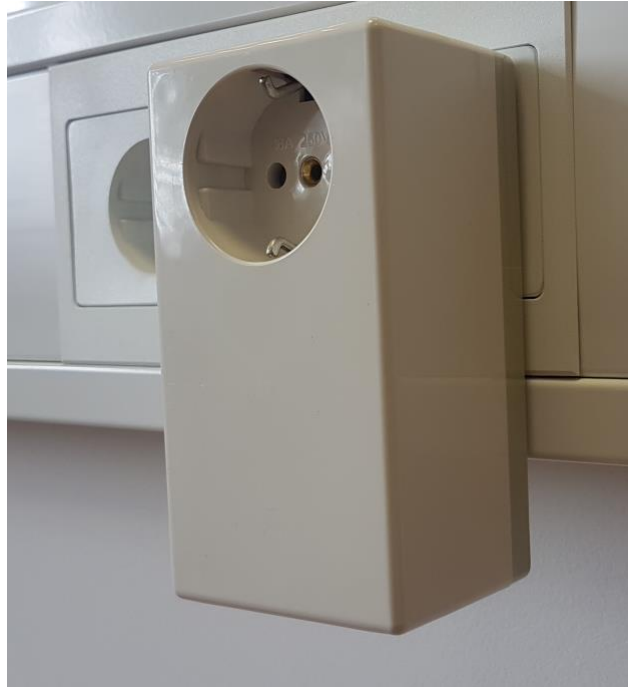
UWB transceiver for indoor localization
