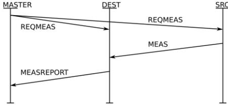
Fig. 6. Channel sounding slot representation.
