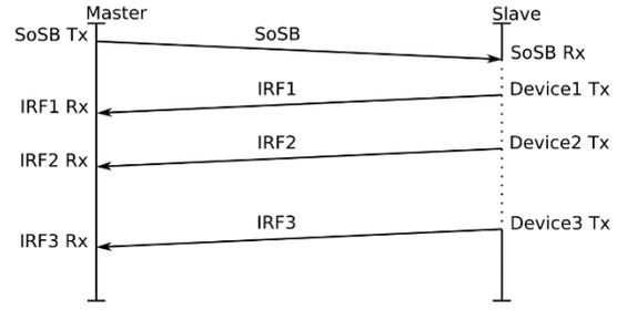
Fig. 4. MGMT slot communication events with one master anchor device, two anchor slave devices and one wearable agent
